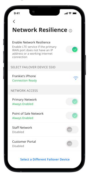
From the My Network screen, tap **Network Resilience** to select a mobile device to provide secondary cellular/LTE service for your most critical networks during internet outages.
