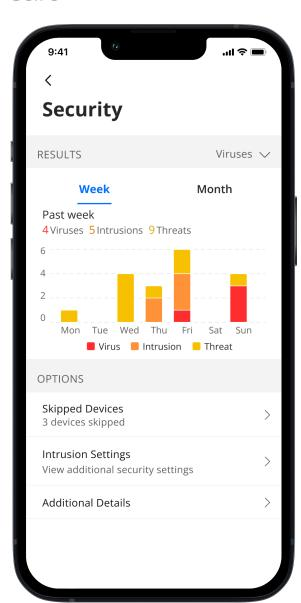
Your router automatically scans data coming into each network for viruses and other malicious content to provide an extra layer of protection against malicious traffic. Threats are automatically blocked from entering the network.
