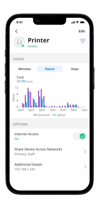
The Device details screen shows the device name at the top of the screen followed by a chart that indicates the amount of data that was used by the device over a period of time.
